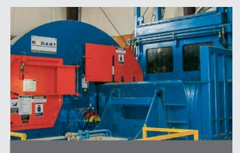
**Disc and ring stranders** cut logs into strands for engineered wood applications including OSB.
