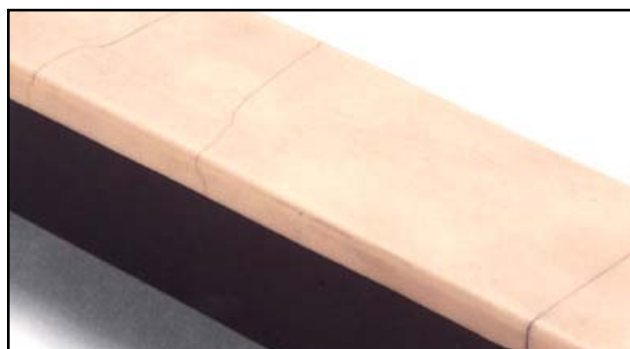
Fig. 19: When exposed to the severe thermal shock felt strips experience, these Al ceramic strips crack. SN stays intact.
