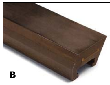
Fig. 9: With female foot designs (A) thermal expansion of the FRP base places the ceramic under stress than can cause cracking. The Kadant AES male foot design (B) eliminates preventable stress concentration points.
