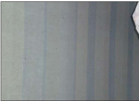
Press fabric streaks due to poor oscillating shower performance.
