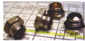
Figure A Nozzles after installation and removal. Note the ungalvanized ArresTech equipped nozzle on the right.
