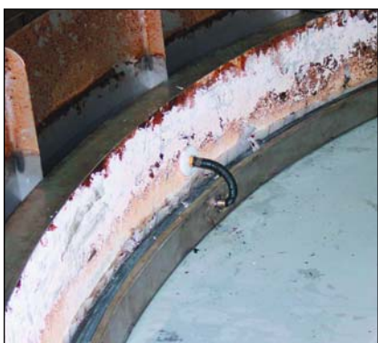
Inflatable gasket on ring and airline connection.
