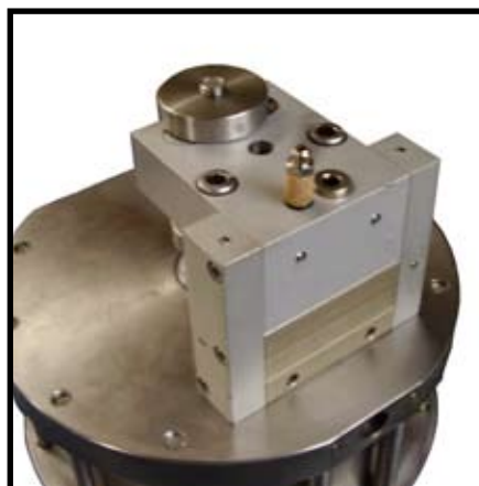
Control valve block with protective cover removed
